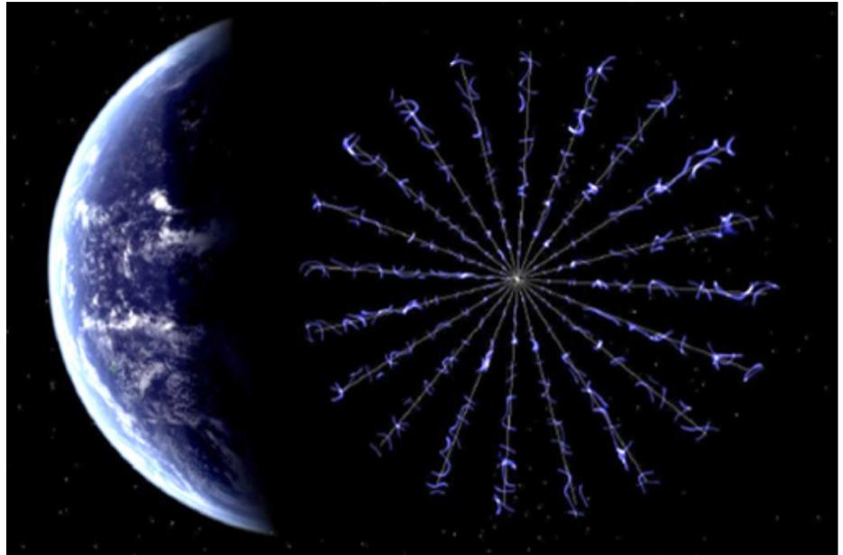
*Long, very thin, bare wires construct this large, circular electric sail. The momentum exchange is produced as protons are repelled by the positively charged wires to create the spacecraft's thrust. Credits: NASA/MSFC.*
