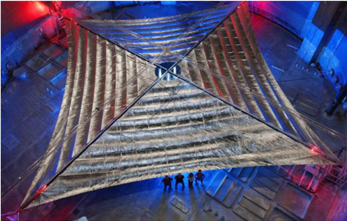
Solar sails are made of ultrathin, highly reflective material. When a photon from the sun hits the mirror-like surface, it bounces off the sail and transfers its momentum. Credit: NASA/MSFC.
